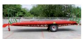
5) 7T low-loading platform for transporting box pallets, height from the ground 88 cm, rigid suspension, open load platform 740 cm x 245 cm/125cm
