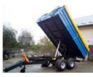
• A system of sideboard tensioning cables with a release bolt Additional wiring system for the second trailer towed
