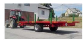
3) 12T stake platform, parabolic TANDEM suspension, height from the ground 118 cm, load platform 900 cm x 250 cm/125 cm
