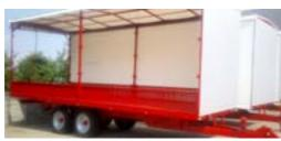
2) 12T low-loading stake platform, height from the ground: 88 cm, rigid suspension, open load-carrying body 600 cm x 250 cm
